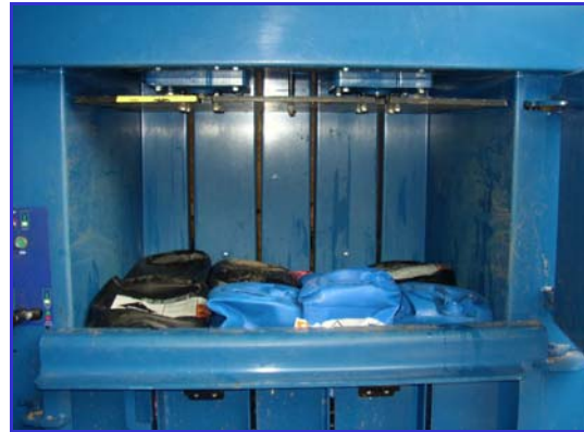
Part-crushed 23-litre containers
